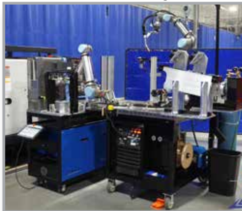
Automated Welding Station
